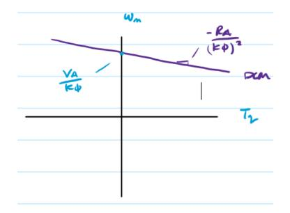
Usually,  $-\frac{R_a}{(k\phi^2)}$  is shallow slope
