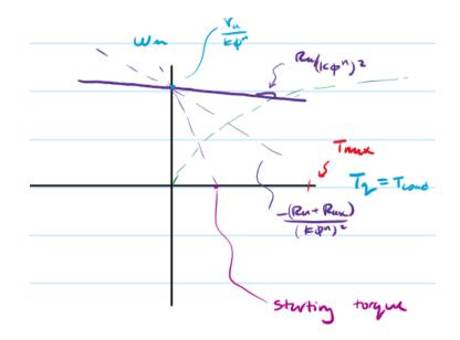
Don't want starting torque  $<< T_{max}$  (torque at 0 speed should not be extremely large)
