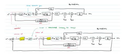
Figure 1: DC Current Control and Speed Control loops
