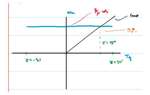
If operating point requires  $\gamma > 90^0$ , machine cannot reach (loss of synchronization).
