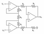
$$= V_2 = V_{CM} \quad V'_1 = V'_2 = V_{CM} \Rightarrow I_G = 0, V_o = 0$$
